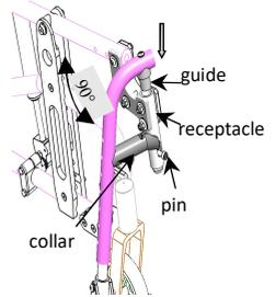
pic. 3.2: Inserting the legrest tube (swing-away version)
