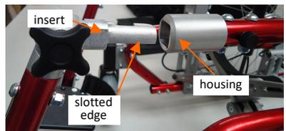
pic. 3.1: Inserting the legrest tube (detachable version)
